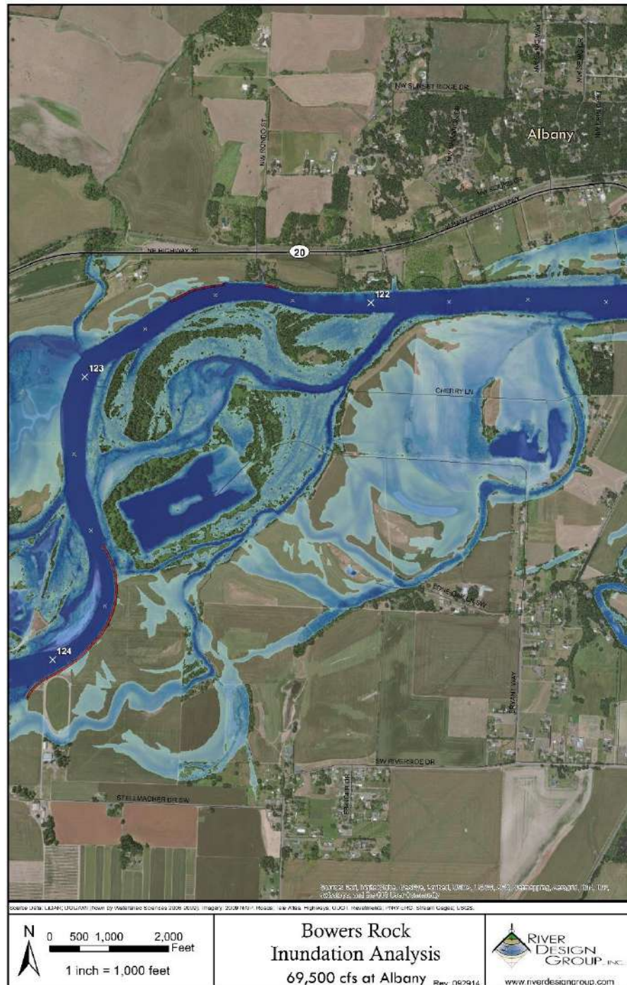
Figure 2-4. The 2-year flow inundation map prepared for BRSP. The modeled inundation level represents a discharge of 69,500 cfs as measured at the USGS gage at Albany, OR.
